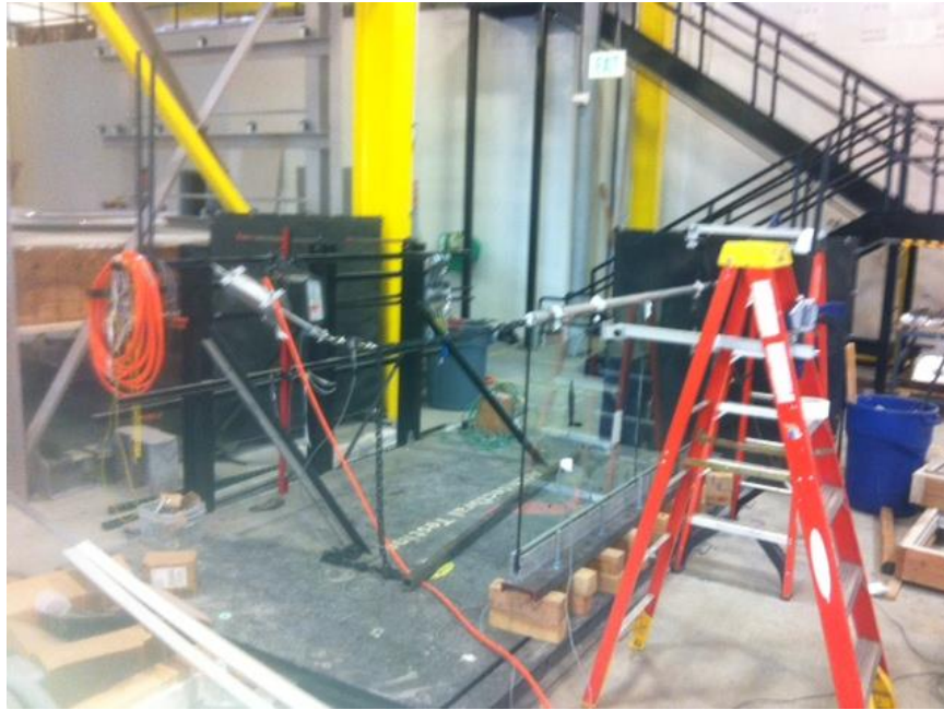
Photo No. 3 Typical horizontal loading deflection setup
